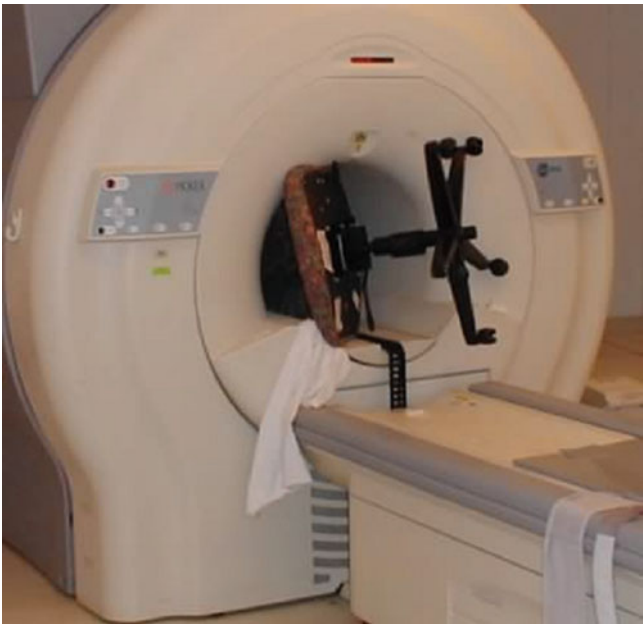
Fig. 33.1 Non-MR conditional chair attracted to magnet
