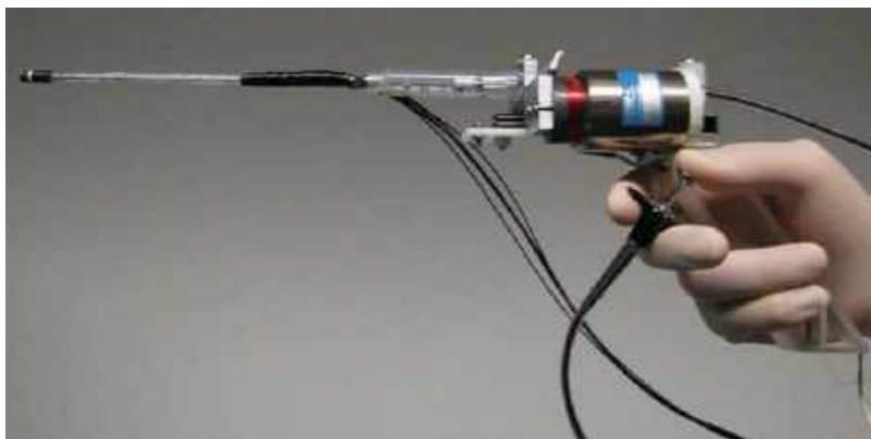
Fig. 69.2 Handheld 1-degree-of-freedom Motion Compensation Instrument
