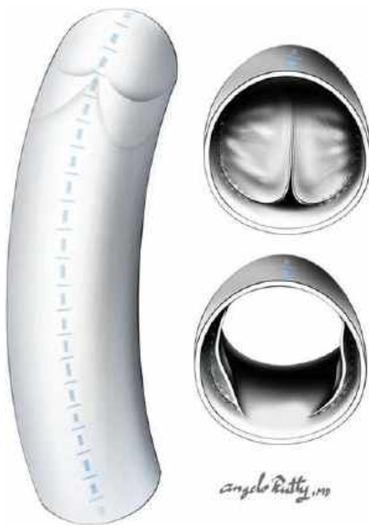
Fig. 100.4 Bicuspid valved PTFE conduit. The valves are constructed from 0.1 mm thick PTFE membranes. There is a small, non-valved opening at the base of the leaflets ( upper right drawing ) to allow minimal regurgitation and prevent thrombosis at the sinuses
