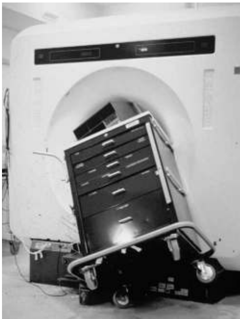
FIGURE 45-5 Magnetic resonance imaging cart that is not compatible inadvertently brought into scanner room.
