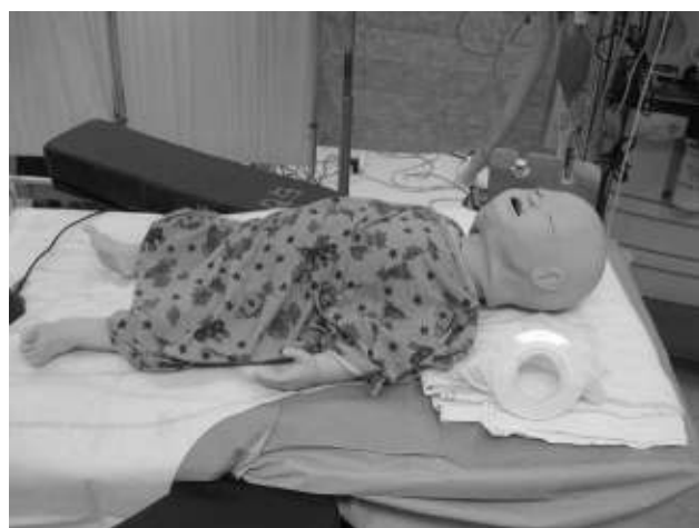
FIGURE 53-2 An infant human patient simulator (Laerdal SimBaby [Laerdal Medical, Stavanger, Norway]) exhibits standard vital signs, variable airway features (tongue swelling, laryngospasm), breath sounds (retraction, wheezing), cardiovascular features (palpable pulses, heart sounds), and others (abdominal sounds, bulging fontanelle).
