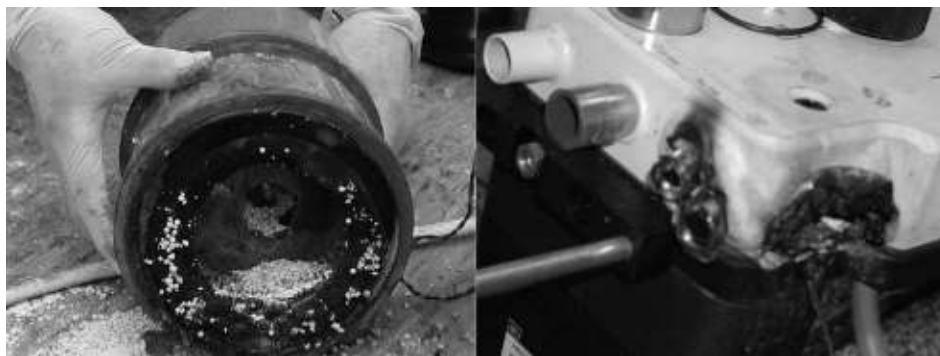
FIGURE 51-8 Sevoflurane/Baralyme interaction produced this fire in an anesthesia machine. (Courtesy Mr. A. Rich.)
